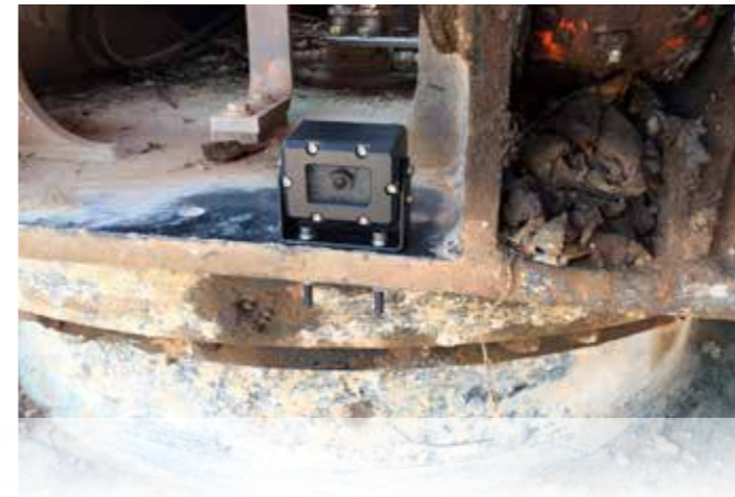
Reversing camera on a road-rail excavator, the MC3000B is shown here.
