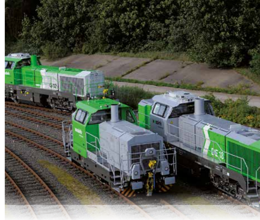
Transport locomotives with 3 or 4 axes: Camera-monitored shunting.
