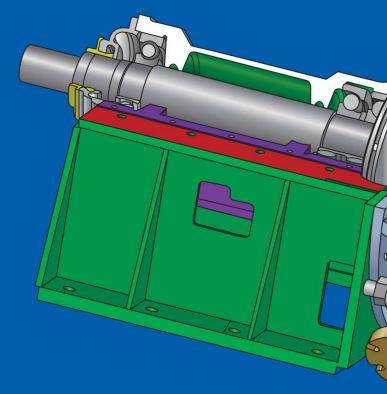
Solids ranging from 19mm to 73mm can be handled. Bearings are selected for a minimum B -10 life of 24,000 hours at maximum speed & impeller diameter. Lubrication of bearings are grease as standard, with oil lubrication available as optional extra. Shaft sleeve fit and impeller hub thread are sealed from pumping media for extended sleeve life.
