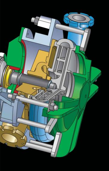
The wet end is manufactured with cast chrome iron CR28% material as standard for increased wear life. The RX range can handle S.G up to 1.3. The RX range can be used in Fly ash, Soda ash, Pot ash and many more applications.
